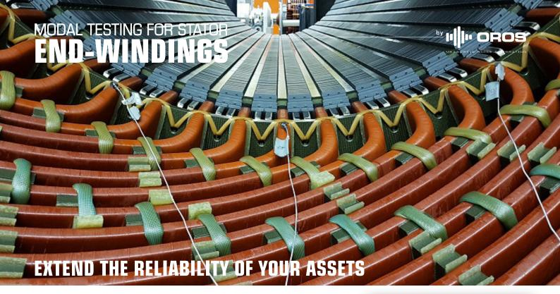
End-winding tests are essential for evaluating the structural integrity and performance of stator windings in large electrical machines. They are invaluable tools in both manufacturing and maintenance contexts.
